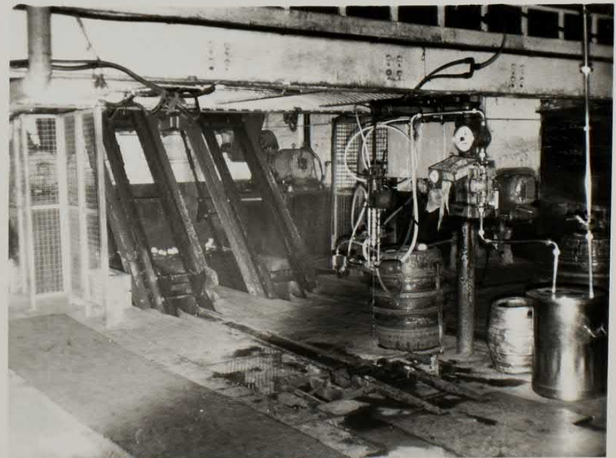
Cask fining machine and cask elevators
