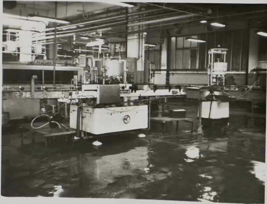
No.5 Line. 'Bulldog' Export. Filler, labeller, crimper.
