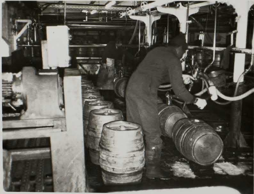
Cask racking line Cask racking , hammering in temporary shives
