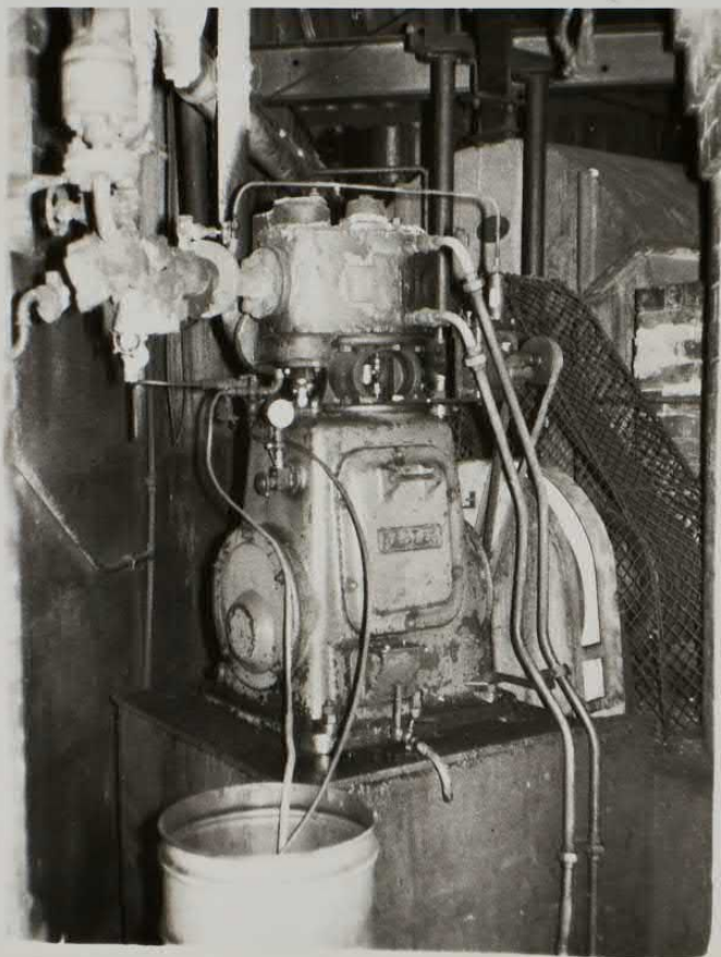
Induced draught fan steam engine, Maker Reader
