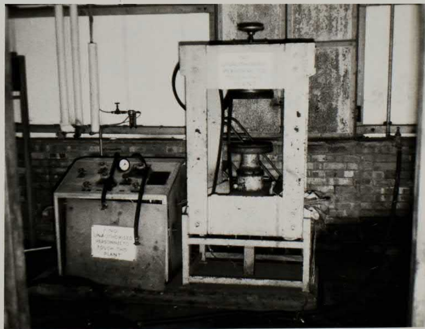
Hydraulic press for cask end repairs
