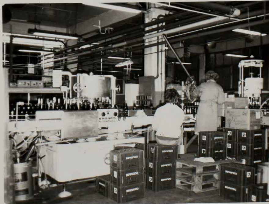
No.5 line. 'Export' Multiseal foil crammer , also filler
