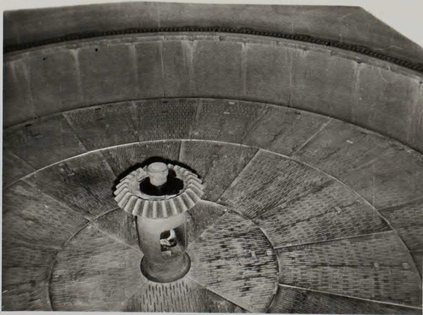
Interior of mash tun showing grid
