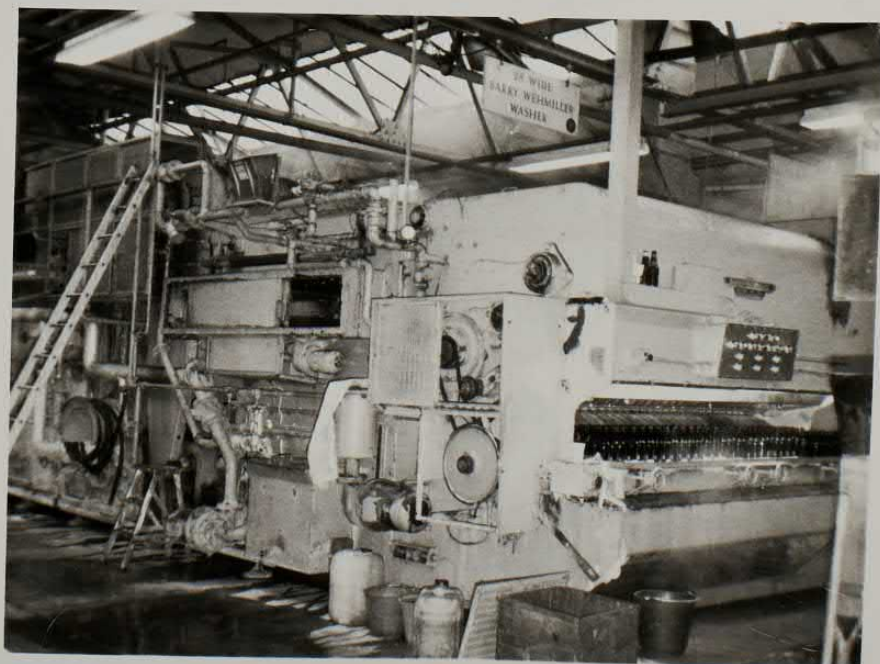
No.1 line. Bottle washing, discharge end
