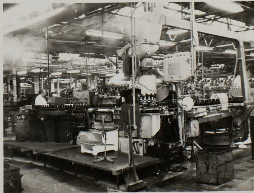
No.1 line. Bottle filler and crown corker
